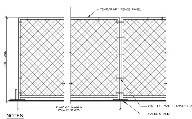
I. WIRE TIES, RAILS POSTS AND BRACES SHALL BE CONSTRUCTED ON THE SECURE SIDE OF THE FENCE ALIGNMENT. CHAIN-LINK FABRIC SHALL BE PLACED ON THE OPPOSITE OF THE SECURE AREA. 2. ALL CHAIN LINK MESH FABRIC TO BE GALVANIZED 72" 9 GAUGE OR HEAVIER WIRE WITH NO LARGER
