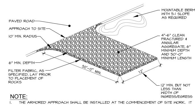
SHALL REMAIN IN PLACE UNTIL THE APPROACH AND SITE ARE PAVED. MATERIAL USED SHALL CONTAIN NO FINES! THIS DETAIL SHALL BE UTILIZED AT ALL APPROACHES ONTO PUBLIC ROADS. APPROACHES SHALL BE MAINTAINED IN A FASHION WHICH PREVENTS SEDIMENT FROM TRACKING/FLOWING ONTO PUBLIC RIGHT-OF-WAY. ADDITIONAL ROCK SHOULD BE ADDED AS NECESSARY. ALL SEDIMENT SPILLED, DROPPED, WASHED, OR TRACKED ONTO PUBLIC
