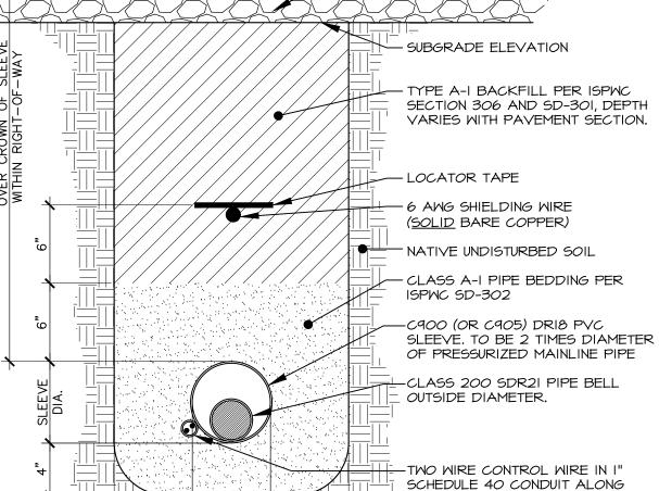
COORDINATE WITH OTHER CONTRACTORS TO INSTALL SLEEVE, CONDUIT, FINDER TAPE AND LOCATING WIRE PRIOR TO INSTALLATION OF ROADWAY IF APPLICABLE.
