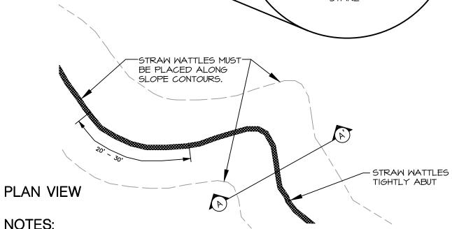
STRAW WATTLES ARE TUBES MADE FROM STRAW BOUND W/ PLASTIC NETTING. THEY ARE APPROXIMATELY 8" DIA. AND 20'-0" TO 30'-0" LONG. STRAW WATTLES TRAP SEDIMENT AND REDUCE SHEET & RILL EROSION BY REDUCING SLOPE GRADIENT, INCREASING INFILTRATION RATES AND BY PRODUCING A
