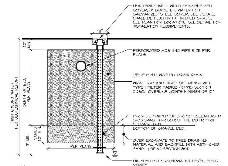
CONTRACTOR SHALL EXCAVATE A TEST PIT AT ALL SEEPAGE BED LOCATIONS TO CONFIRM THE DEPTH TO FREE DRAINING SOILS AND GROUNDWATER IN THE PRESENCE OF THE LANDSCAPE ARCHITECT PRIOR TO CONSTRUCTION.
