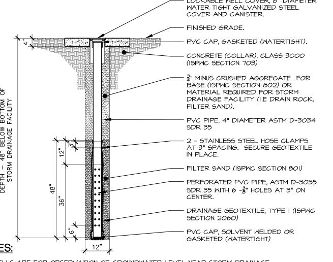
I. WELLS ARE FOR OBSERVATION OF GROUNDWATER LEVEL NEAR STORM DRAINAGE FACILITIES.
