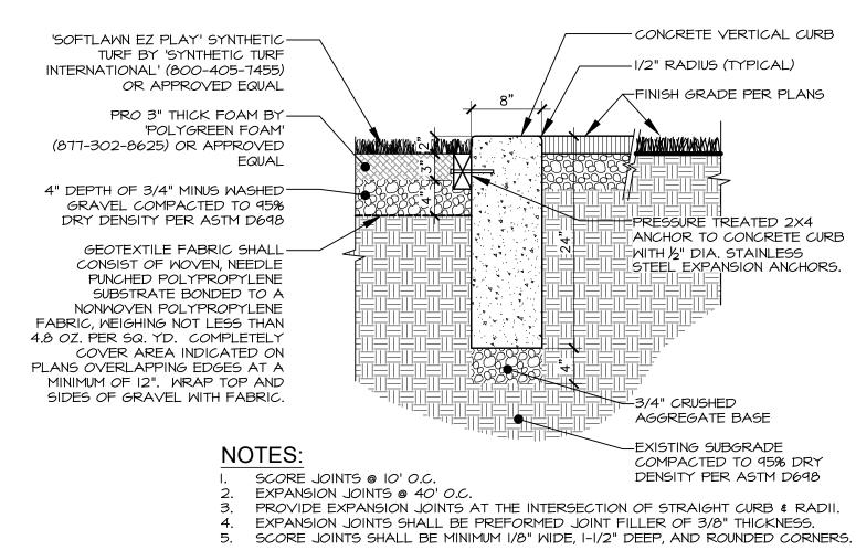
SYNTHECTIC TURF SURFACING ALT 4C AND 4F Scale: 1"= 1"-0"
