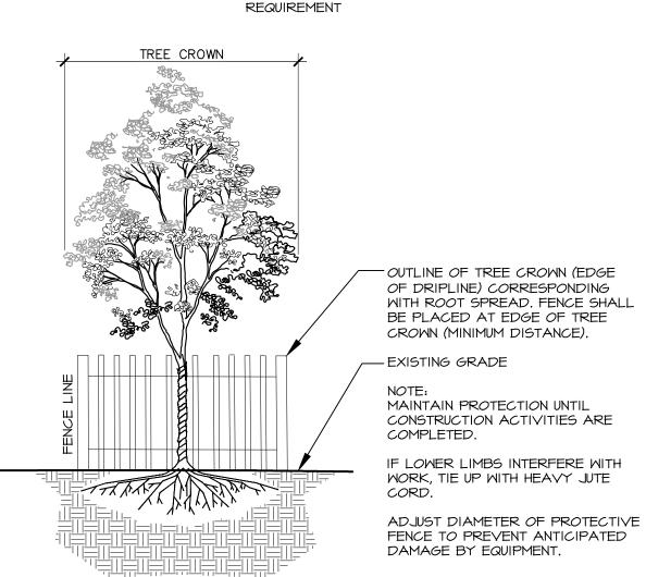
TREE TRUNK - CROWN OF TREE. - OUTLINE OF TREE CROWN (EDGE OF DRIPLINE) CORRESPONDING WITH ROOT SPREAD. FENCE SHALL BE PLACED AT EDGE OF TREE CROWN (MINIMUM DISTANCE).
