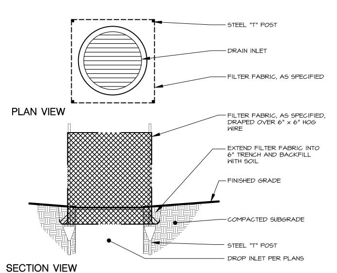
INSPECT PERIODICALLY AND REPAIR/REPLACE AS REQUIRED. REMOVE SEDIMENT ACCUMULATIONS WHEN FILTER CAPACITY IS IMPAIRED. OTHER METHODS OF INLET PROTECTION MAY BE APPROVED UPON REVIEW BY THE LANDSCAPE ARCHITECT.
